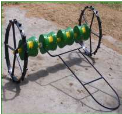
Figure 1. Eight row paddy seeder. (Courtesy: M/s. KSNM Marketing, Coimbatore, India)
