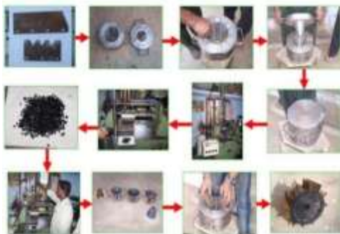
Figure 3. Production process of plastic moulded Cono weeder (Courtesy M/s. KSNM Marketing, Coimbatore, India)
