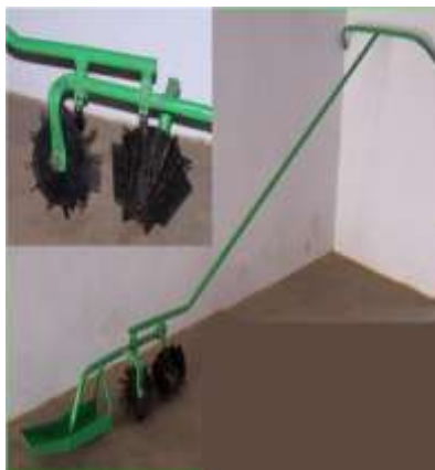
Figure 2, Plastic moulded cono weeder. (Courtesy: M/s. KSNM Marketing, Coimbatore, India)
