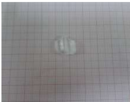
Figure 1.c. KNO 3 doped L-arginine single crystal (3:1)
