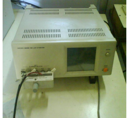
Figure 1 Dielectric spectroscopy [LCR HITESTER 3532-50]
