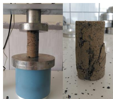
Figure 3. Injected granular soil samples; (a) under the unconfined compressive test and (b) after the unconfined compressive test
