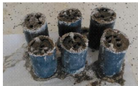
Figure 2. Injected granular soil samples
