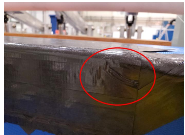
Figure 2. Wrinkles appear on uncured composite laminates
