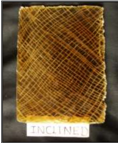
Figure 2.3. Inclined oriented PALF reinforced composites
