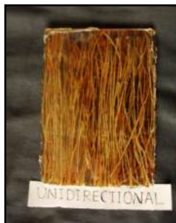
Figure 2.1 Uni-directional oriented PALF reinforced composites
