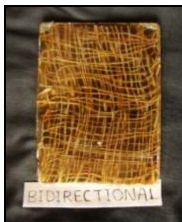
Figure 2.2. Bi-directional oriented PALF reinforced composites
