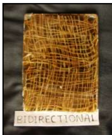
Figure 2.2. Bi-directional oriented PALF reinforced composites
