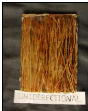
Figure 2.1 Uni-directional oriented PALF reinforced composites
