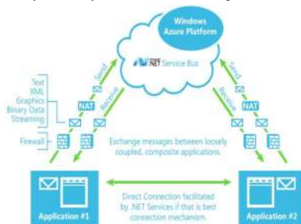
Fig. 8 Service Bus Access Control
