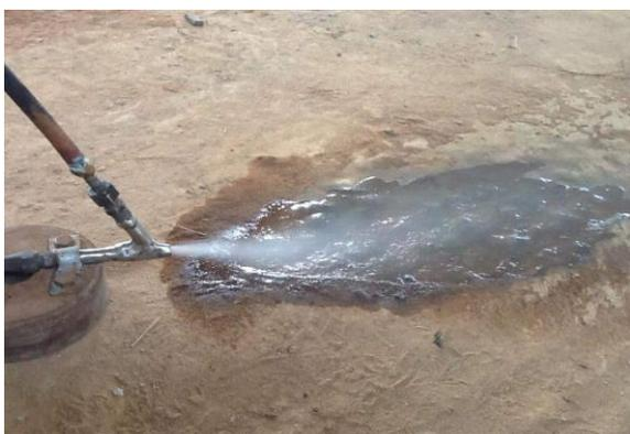
Figure 7: Spray for  $\alpha = 60^\circ$  and  $\Delta P = 3$  bars.
