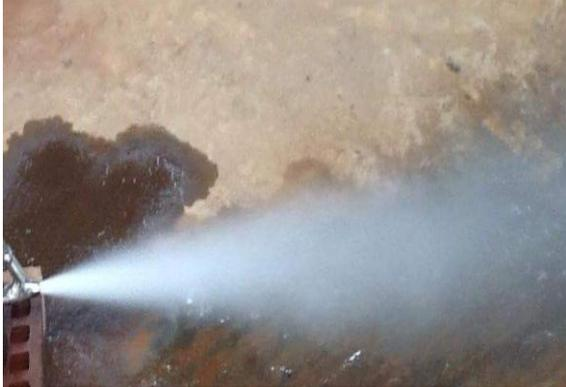
**Figure 11: Spray for  $\alpha = 60^\circ$  and  $\Delta P = 15$  bars.**
