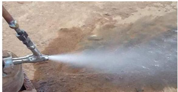
Figure 9: Spray for  $\alpha = 60^\circ$  and  $\Delta P = 9$  bars.
