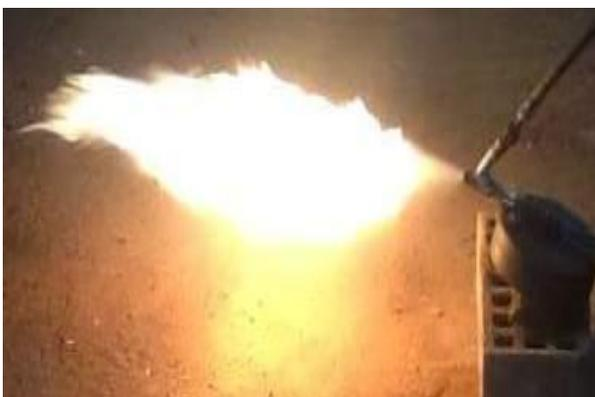
**Figure 12: Flame for  $\alpha = 60^\circ$  and  $\Delta P = 3$  bars.**
