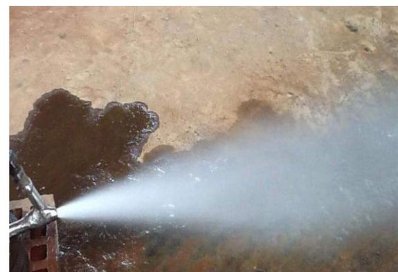
Figure 10: Spray for  $\alpha = 60^\circ$  and  $\Delta P = 12$  bars.
