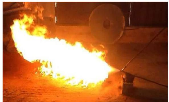
**Figure 15: Flame for  $\alpha = 60^\circ$  and  $\Delta P = 12$  bars.**
