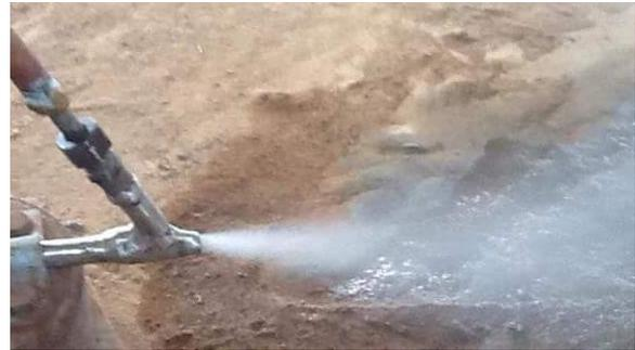
Figure 8: Spray for  $\alpha = 60^\circ$  and  $\Delta P = 6$  bars.
