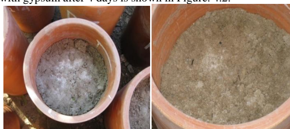
Figure. 4.2. Appearance of Salt Crystal (Na 2 SO 4 ) from Soil after Gypsum Treatment
