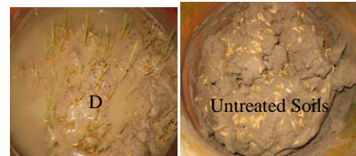
Figure 4. ( a ) Testing of Rice Plant Growth in the Gypsum Treated Soil and Untreated Soil (5 days)
