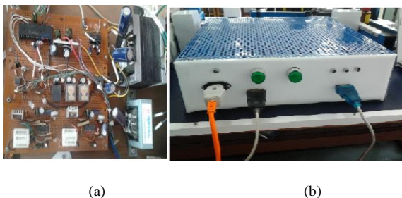
Figure 7. (a)Electrical Setup and (b) Control box
