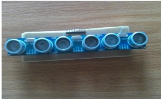
Plate 6 Implementation of Sensor Unit on Printed Circuit Board
