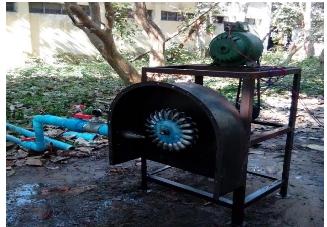
Figure 11. Assembly of Pelton Turbine
