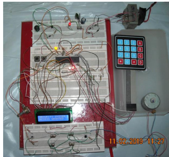
Figure 13. Experimental testing of the code-protected door control system
