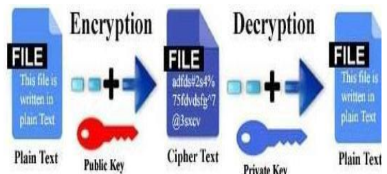
Figure 2.2: Encryption and Decryption (Jaydip, 2019)
