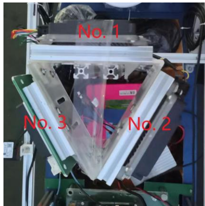
Figure 1. Millimeter wave radar installation
