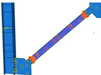
Figure 10. Connection of Steel Central Core and Concrete Cover of the Buckling-Restrained Moment Frame with Tie Constraint.
