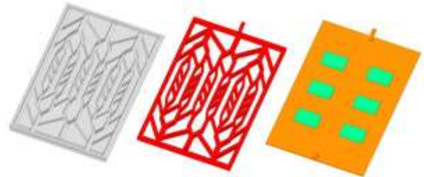
Figure 1 IGBT Liquid Cooling Channel Model
