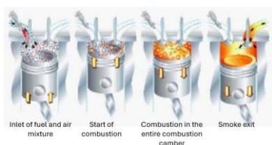
Figure 1: Stages of the homogeneous mixture compression ignition engine cycle
