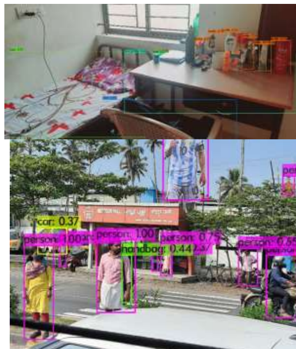
Fig.7. Real-time item detection in the room
