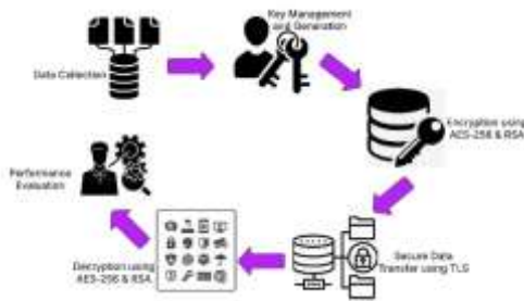
Figure 1: Enhanced Data Security with Hybrid AES-256 and RSA Encryption for Secure Transmission and Storage
