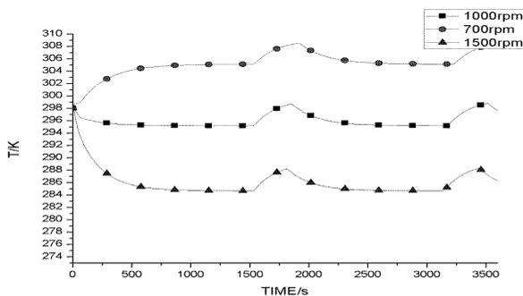
Figure.18. Influence of compressor speed on heat dissipation of motor
