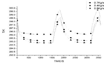
Figure.16 Influence of air flow on heat dissipation of motor
