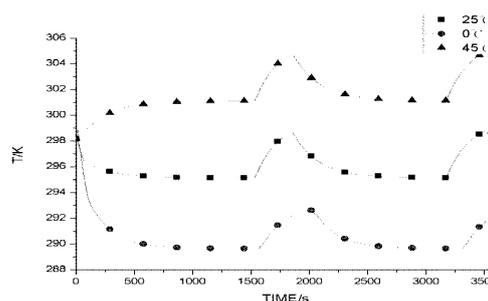
Figure.14 Influence of outdoor temperature on heat dissipation of motor
