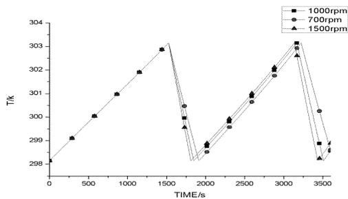
Figure.17 Influence of compressor speed on battery heat dissipation
