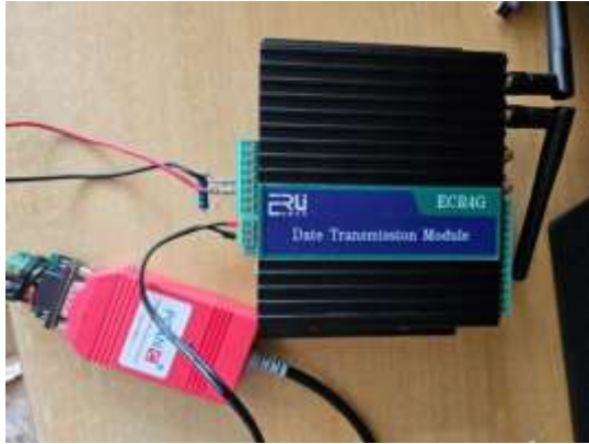
Figure 5. Laboratory connection of the PCAN interface and data-transmission module.
