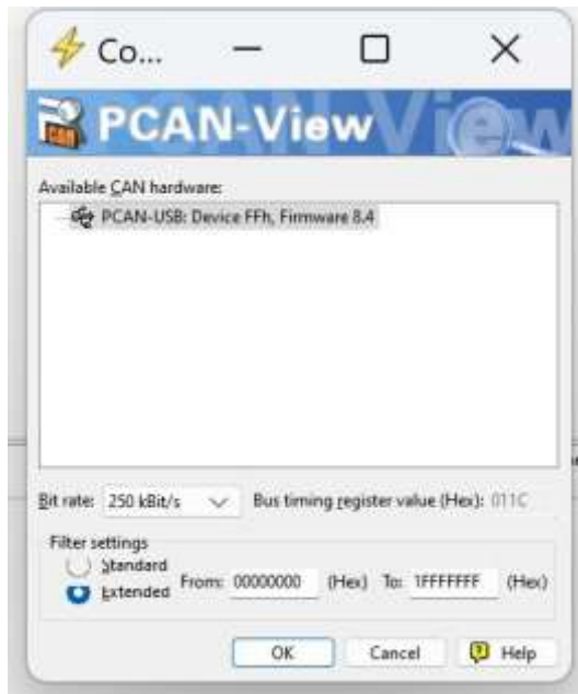
Figure 6. PCAN-View connection and frame-format configuration.
