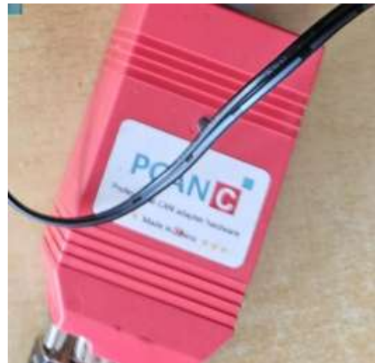
Figure. 4. PCAN-USB interface used to generate simulated CAN traffic.
