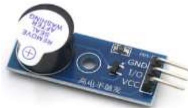
Figure. 7 Low-power high-level triggered buzzer
