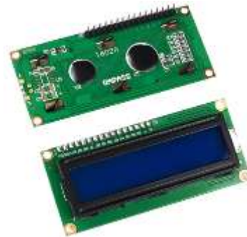
Figure. 6 LCD1602 Liquid Crystal Display
