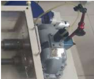
Figure. 2 Gear box lubricating oil circulation device
