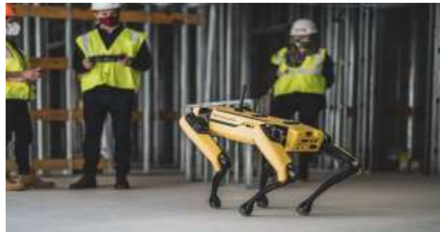
Figure 5: Robotic Site Inspection
