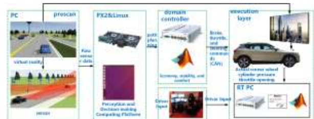
Figure 1 Autonomous driving hardware-in-the-loop platform framework
