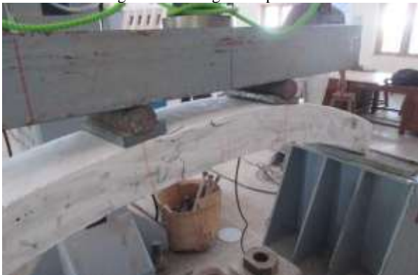
Fig .8 Beam after Loading
