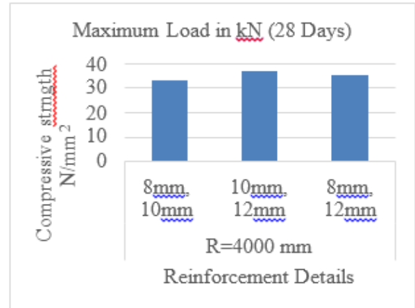
Fig. 9 Compressive strength of curved beams of initial curvature R=4000mm
