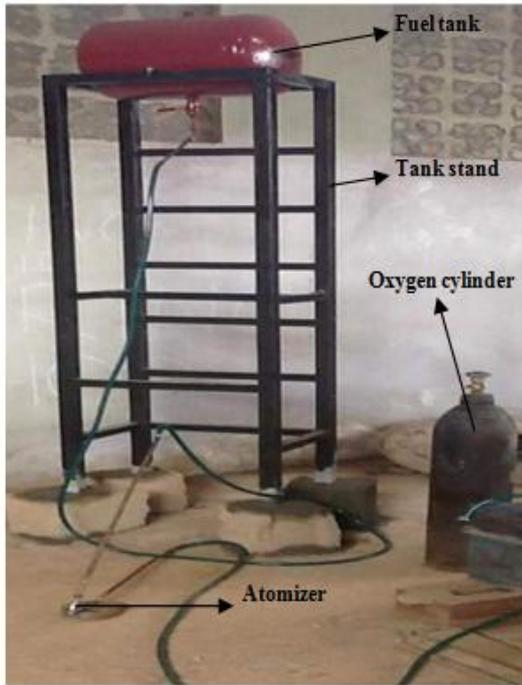
Figure 6: Complete assembly of the system [6].
