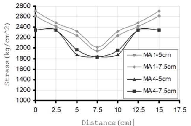
Figure 5: Stress distribution within the width of the beam flange.
