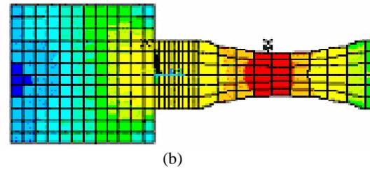
Figure 8: (a) MB5 stress counter, and (b) MB7 stress counter.
