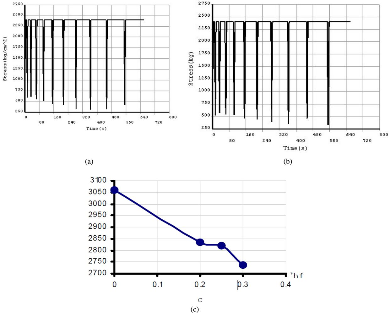
Figure 11: (a) MC2 stress-time curve, (b) MC3 stress-time curve, and (c) stiffness versus c parameter.
