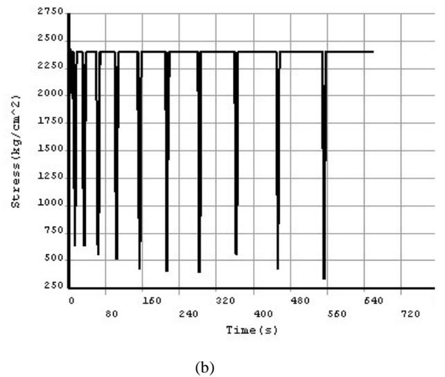
Figure 4: (a) MA1 stress-time curve, (b) MA2 stress-time curve.
