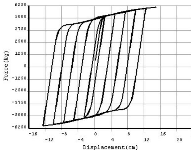
Figure 3: MA2 load-displacement curve.
