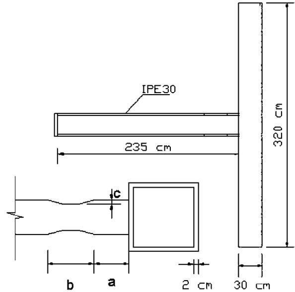
Figure 1: Geometry of RBS connection used in the analytical
