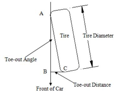
Figure 1. Toe out of tire
