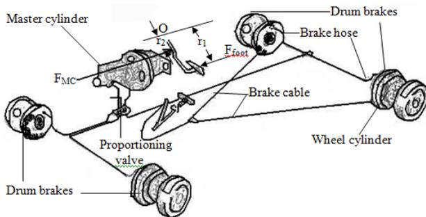
Figure 4. Layout of Hydraulic Pipe Lines
