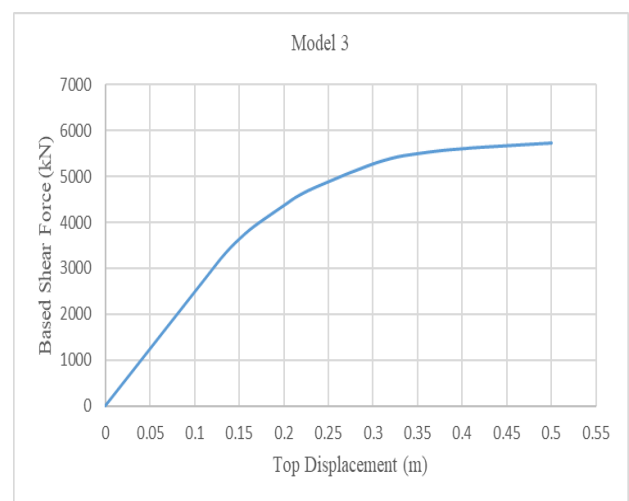
Figure 13. Capacity curves for Y direction by pushover analysis for Model 3.
