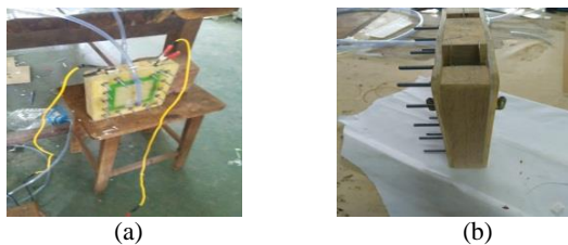
Figure 3.1 (a) Finished Electrolyser with Bubbler (b) Hydrogen Dry Cell
