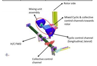
**Torque tube and lever assembly:** The pilot limit loads during jamming conditions are shown in Figure 2. A factor of safety of 1.5 is used over these loads and these loads are applied to the torque tube and lever assembly FE model.
