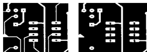
Binary image f f \circ s (5x5 square) Figure 2 Results of Opening with a Square Structuring Element [11]
