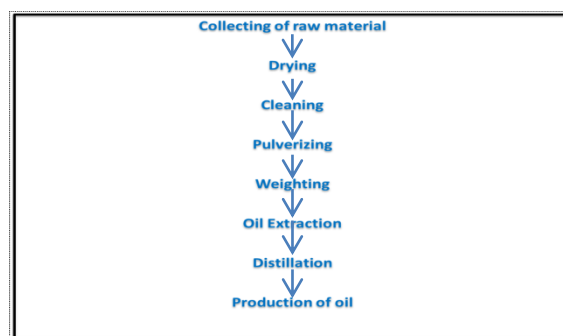
Figure 2. Flow chart of Extraction of oil from algal biomass
